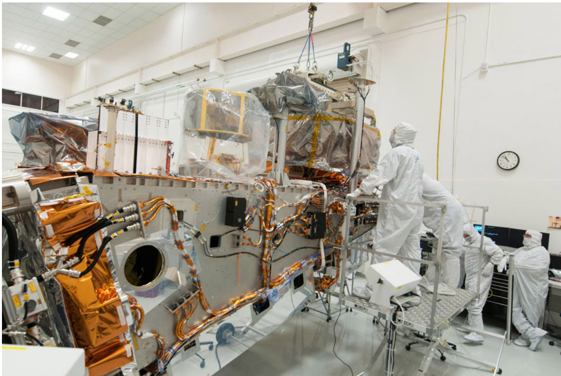
Caption: Ball and Raytheon technicians integrate the VIIRS Optical and Electrical Modules onto the JPSS-1 spacecraft in 2015. The spacecraft will be ready for launch later this year. Image Credit: Ball Aerospace & Technologies Corp.
